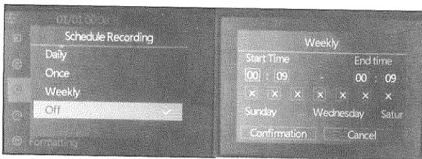
On the above menu, the device allows you to set up a daily recording, a one time recording, or a weekly recording.
